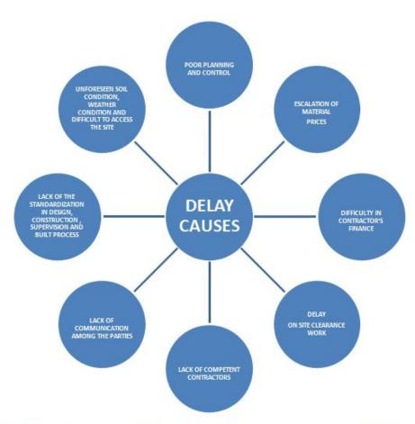
Eight main delay causes (Delay factors) in the Dungquat refinery project of Vietnam
