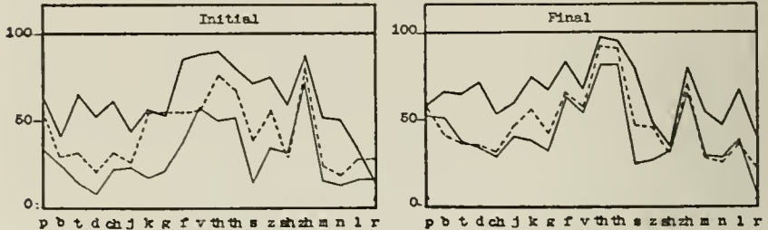
Plate XLIX.—Per cent of Substitution for the respective Simple Consonantal Sounds heard through the dictaphone (upper solid line), telephone (dotted line), and the air (lower solid line). (The second th is vocalized; elsewhere represented by dh ).
